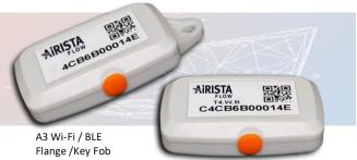
AiRISTA's A3 asset tag is designed to monitor assets within a Wi-Fi / BLE network environment. The A3 Wi-Fi / BLE asset tag provides options to generate alerts based on vibration.
